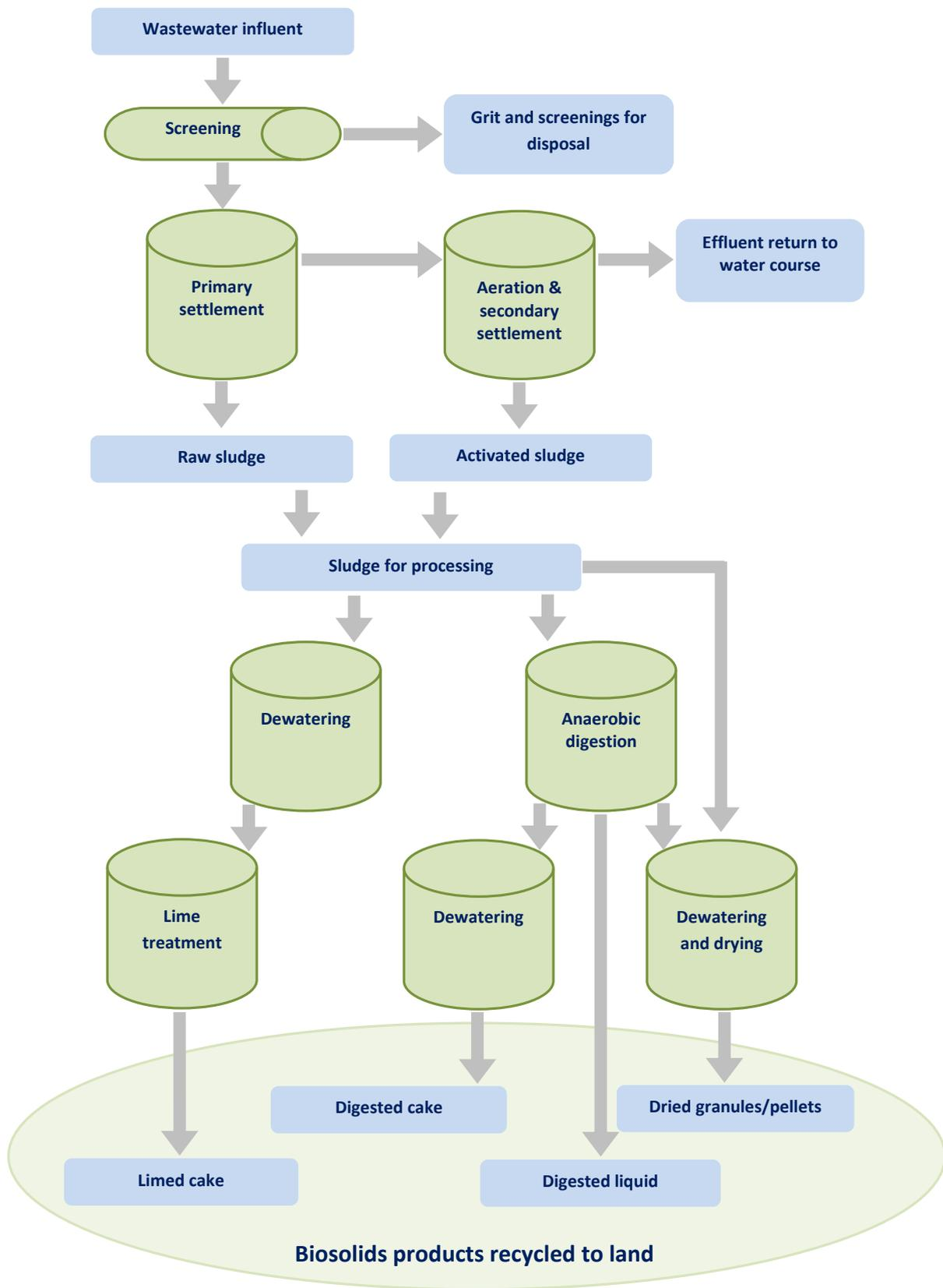
**Figure 1. A typical process flow from wastewater influent to biosolids products**
